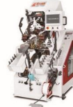
带电脑自动上胶前帮机(九爪) Computerized toe lasting machine with cementing (9-pincer)
