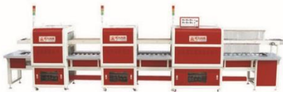
标准电路控制双层红外线贴底开发室生产线(单边式) Double-layer outside Cementing and Assembling Conveyor (one-side working station)
